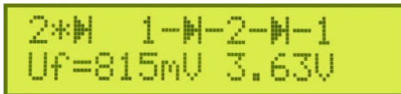
Measuring zener diodes with a zener voltage up to 3.9 V with the MK-168.
